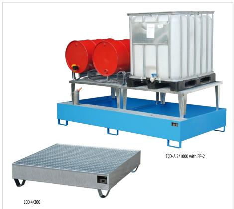
Max. no. of Dimensions **Retention capacity** Weight 200 litre drums/1000 litre IBCs in mm (I x w x h) in I painted / galv. in kg ECO 1/200 1/-800 x 800 x 455 222 44/46 ECO 2/200 2/-1200 x 800 x 360 240 54/57 ECO 4/200 4/-1200 x 1200 x 285 261 68/71 ECO 4/400 4/-1200 x 1200 x 410 435 77/80 ECO 1/1000 -/1 1460 x 1460 x 620 1100 141 / 147 ECO 2/1000 -/2 2650 x 1300 x 435 1128 185 / 195 ECO-A 1/1000 1460 x 1460 x 1085 150 / 158 -/1 1100 233 / 244 ECO-A 2/1000 -/2 2650 x 1460 x 865 1128
