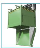
Containers emptied via a trap door are compact in design but also high capacity. An optimised load centre means maximum utilisation of the forklift load capacity. A pull cable operates the base which opens wide; thanks to the large aperture the load is fully discharged every time - even bulky materials.
