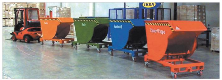
BKM with castors, trailer coupling and towing bar
