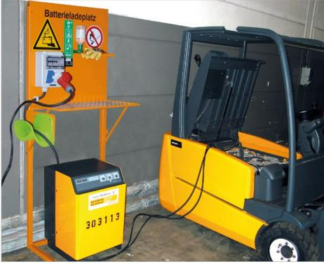
BL with CEEform socket 400 V charging the battery of an electric forklift truck
