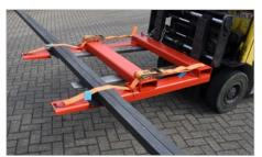
Position: load at the front for loading and unloading
