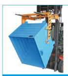
These containers are an economical alternative as they do not have a built-in emptying mechanism. Any number of containers – providing they are the same width – can be picked up by one and the same traverse. Containers without pins must be discharged using a forklift rotator.
