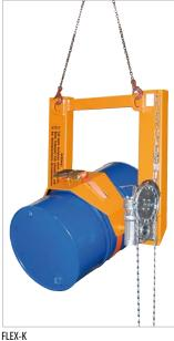
A multifunctional unit - used for transporting, controlled emptying, turning over and setting down drums and other receptacles. Suitable for steel bunghole drums, steel drums with a lid, steel rolling hoop drums, plastic L-ring drums and plastic double L-ring drums ranging from 60 to 220 litres and for 120/240 litre waste bins
