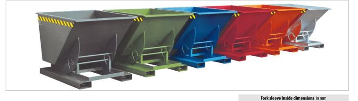
Load capacity Volume Weight Dimensions (approx.) in m<sup>3</sup> in mm (I x w x h) in kg in kg (painted/galv.) AK 50 169 / 182 0,50 1420 x 1008 x 1070 1000 AK 75 0,75 1420 x 1190 x 1070 1000 187 / 202 AK 100 1,00 1420 x 1560 x 1070 1000 218/235 B C A AK 150 1,50 1420 x 2280 x 1070 1000 262 / 282 AK 50-150 600 200 91
