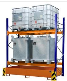
PR Set No. 3 for max. 4 x 1000 litre IBC consists of the following components: 2 x Upright Frame PR-S 3000 4 x Cross Beam PR-T 2700-2 2 x Retainer Bar PR-D 2700 1 x Shelf Sump RW 2700-3 2 x Corner Guard (accessory)
