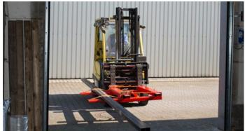
Use the LSL for long material and easily pass through gates or navigate narrow aisles
